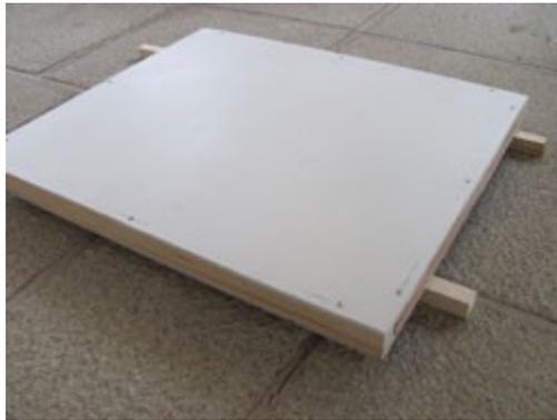
On the top is a layer of fire board, the bottom is a plywood panel and the sandwich is 4 x ¾ inch battens.
